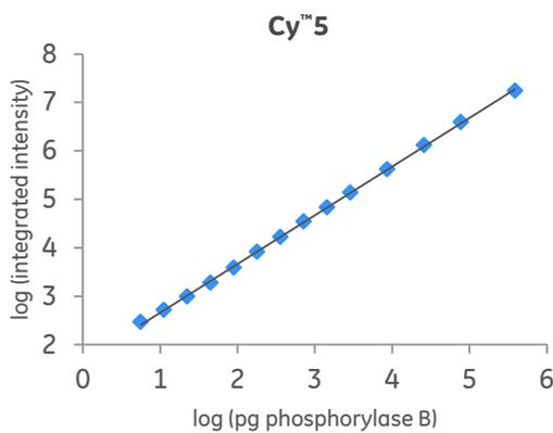
**Fig. 1.** Phosphorylase B was labeled with CyDye™ DIGE fluor Cy5 minimal dye and separated using the Amersham WB electrophoresis gel. The gel was imaged with Amersham Typhoon using normal scan speed. The detection limit was 5.6 pg and the linear dynamic range (DR) was 4.8 orders of magnitude.
