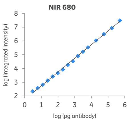
**Fig. 3.** Antibody conjugated with IRDye™ 680 was separated using the Amersham WB electrophoresis gel. To reduce noise, the gel was imaged with Amersham Typhoon using slow scan speed. The detection limit was 3 pg and the linear dynamic range (DR) was 5.2 orders of magnitude.
