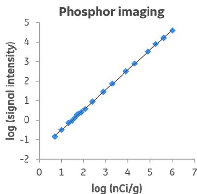
**Fig. 6.** Scanned image of a  $^{14}\text{C}$  autoradiographic standard using Amersham Typhoon. The linear dynamic range (DR) was 5.3 orders of magnitude.
