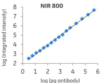
**Fig. 4.** Antibody conjugated with IRDye™ 800 was separated using the Amersham WB electrophoresis gel. To reduce noise, the gel was imaged with Amersham Typhoon using slow scan speed. The detection limit was 3 pg and the linear dynamic range (DR) was 5.2 orders of magnitude.
