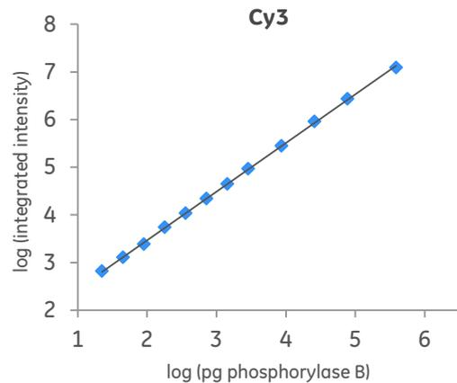
**Fig. 2.** Phosphorylase B was labeled with CyDye DIGE fluor Cy3 minimal dye and separated using the Amersham WB electrophoresis gel. The gel was imaged with Amersham Typhoon using normal scan speed. The detection limit was 22 pg and the linear dynamic range (DR) was 4.2 orders of magnitude.
